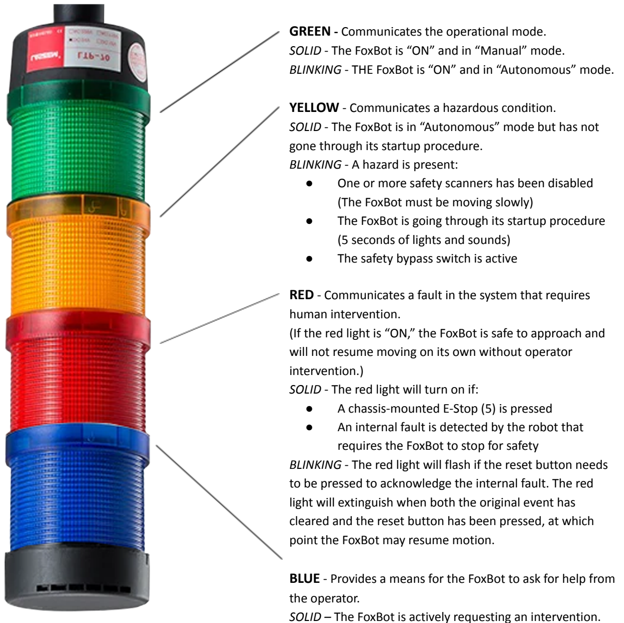
Figure 15 - Typical Stack Light Color Codes
